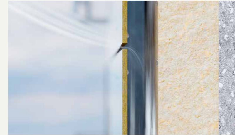
The ventilation effect through behind and through the joint of the cladding
