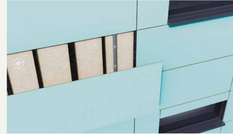
Ventilated facade construction can be demounted individually, which enables reusing and/or recycling them
