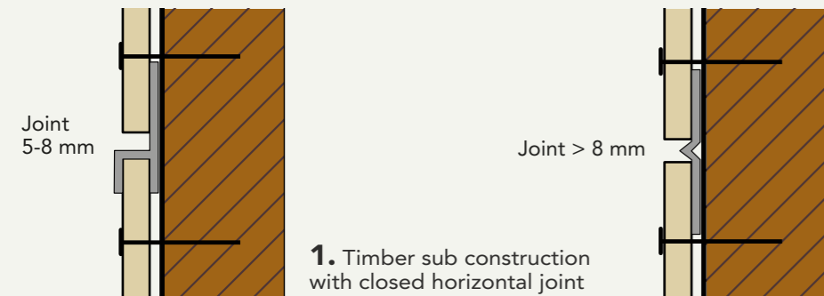
2. Timber sub construction with semi-closed horizontal joint
