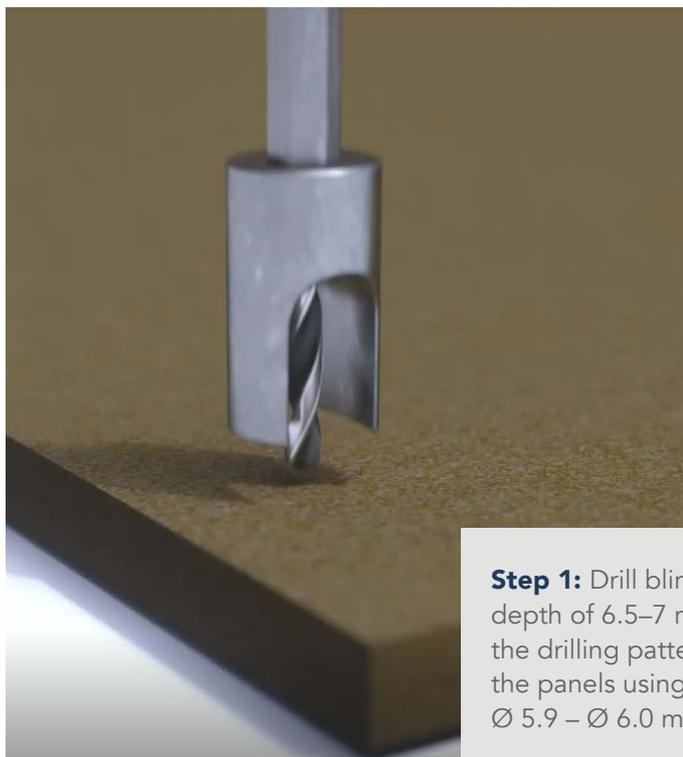
**Step 1:** Drill blind holes to a depth of 6.5–7 mm according to the drilling pattern. Fit clips to the panels using TU-S Diameter:  $\varnothing$  5.9 –  $\varnothing$  6.0 mm.
