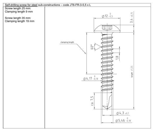
Table 8c - Specifications mechanical fixings - Self drilling screw for steel
