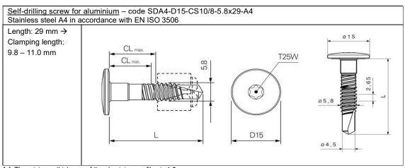
Table 8b - Specifications mechanical fixings - Self-drilling screw for aluminium
