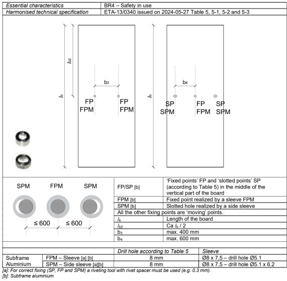
Table 6b – Performance fixings according to table 4 and 5 with the required edge distances, maximum distances and vertical installation of boards.
