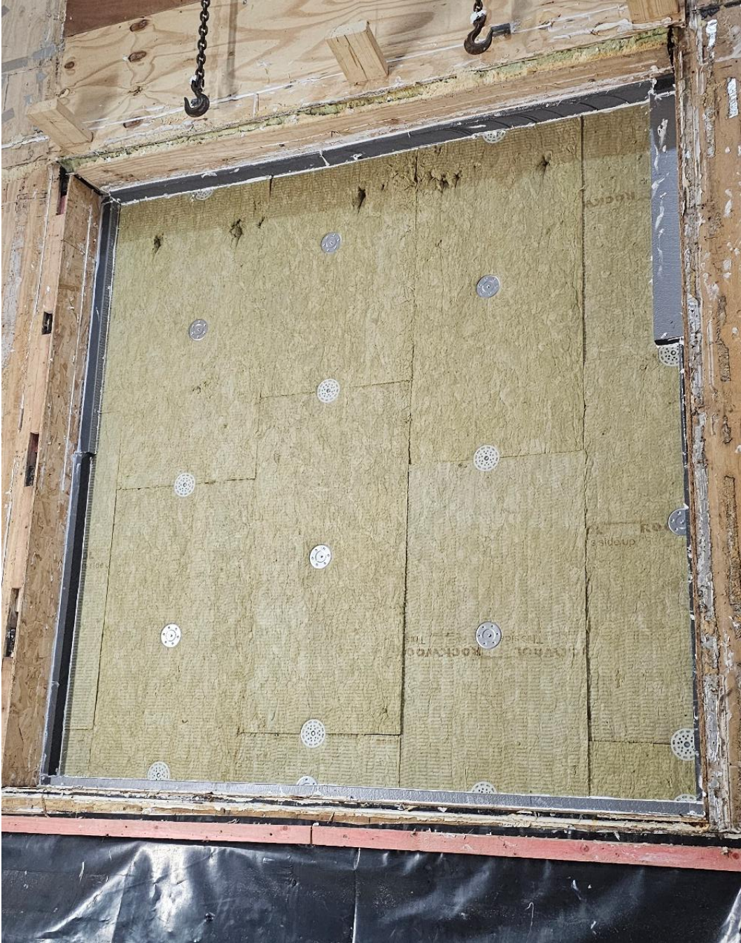
Plate 1 – Sample Sealed Into CWCT Chamber
